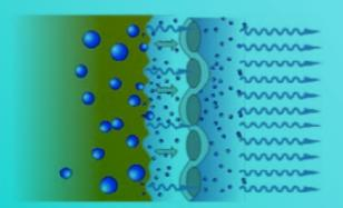
The DMM technology produces a controlled balance and evaporates moisture both on skin and from the outside of the textile.
